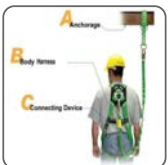
Install/fit fall protection equipment (fall restraint and fall arrest devices)
